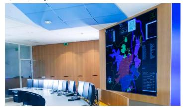
eyevis attached much importance on the possibility to use their cubes even in critical ambient light conditions or other challenging safety-related problems. The **SXGA** version uses a 1-chip-DLP® projector with a display resolution of **1280 x 1024 pixels**.
