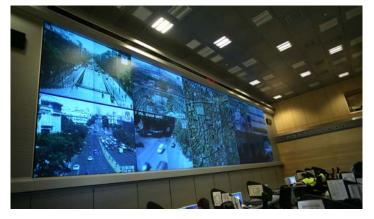
eyevis attached much importance on the possibility to use their cubes even in critical ambient light conditions or other challenging safety-related problems. The XGA version uses a 1-chip-DLP® projector with a display resolution of **1024 x 768 pixels**.
