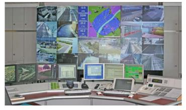
eyevis attached much importance on the possibility to use their cubes even in critical ambient light conditions or other challenging safety-related problems. The SXGA+ version uses a 1-chip-DLP<sup>®</sup> projector with a display resolution of **1400 x 1050 pixels**.
