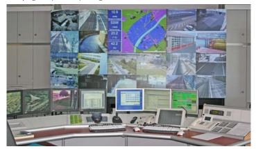
eyevis attached much importance on the possibility to use their cubes even in critical ambient light conditions or other challenging safety-related problems. The SXGA+ version uses a 1-chip-DLP® projector with a display resolution of 1400 x 1050 pixels.
