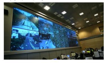
eyevis attached much importance on the possibility to use their cubes even in critical ambient light conditions or other challenging safety-related problems. The XGA version uses a 1-chip-DLP® projector with a display resolution of **1024 x 768 pixels**.
