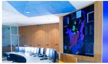
eyevis attached much importance on the possibility to use their cubes even in critical ambient light conditions or other challenging safety-related problems. The **SXGA** version uses a 1-chip-DLP<sup>®</sup> projector with a display resolution of **1280 x 1024 pixels**.
