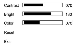
Use the + and – buttons to choose the desired parameter, press Menu to select and then use + or – to increase or decrease the value. Press Menu to save the value. When finished with all adjustments, use the + and – buttons to move to Exit and then press Menu to actually exit the routine.
